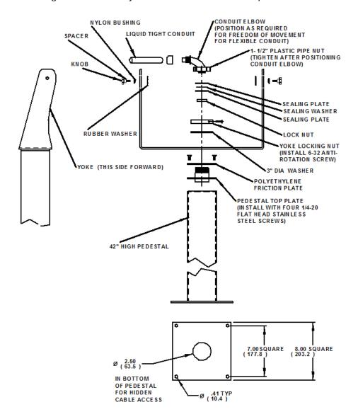
**Note**: The ¾" conduit and other sealing hardware are not required for NEMA 12 monitors or NEMA 4/4X monitors with the 4-cable gland.
