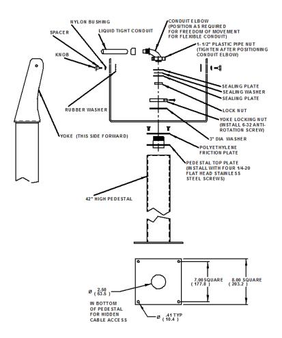
Note: The ¾" conduit and other sealing hardware are not required for NEMA 12 monitors or NEMA 4/4X monitors with the 4-cable gland.
